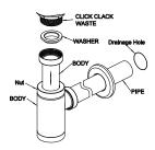
Step2: Loosen the nut, and then pull the body to adjust up and down, so that the outlet of the body is in line with the drainage hole. Insert the pipe into the drainage hole, put the washer into the body, install it on the click clack basin waste, and then tighten the seal.
