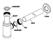
Disassemble all the parts according to the figure above. Please note that Parts are for illustrative purposes only and may differ slightly to the actual product
